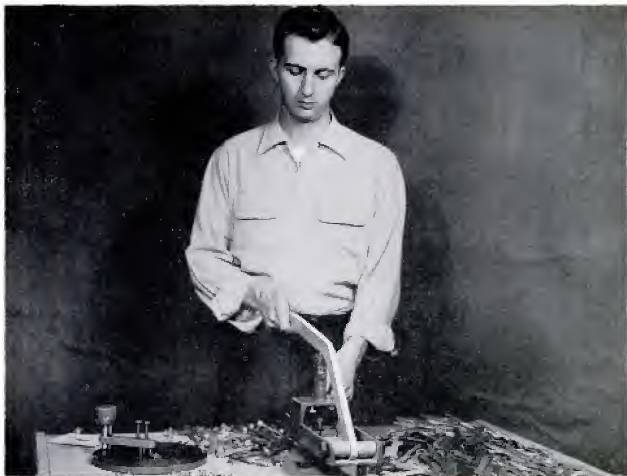
Perrine notches sheared strips in last step of punching process. Finished strips at left are ready for bending
